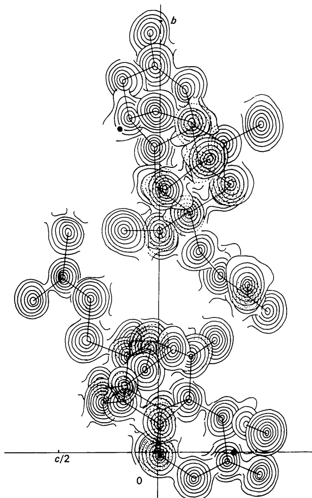
Fig. 3. The final composite Fourier map projected along the a axis, contours being drawn at intervals of 1 e.Å -3 . Contours for the iodine atoms are omitted and their positions are shown with black circles.
